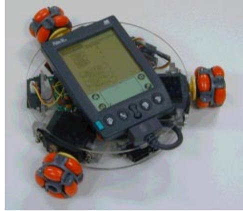
**Figure 6:** The Palm Pilot Robot Kit
